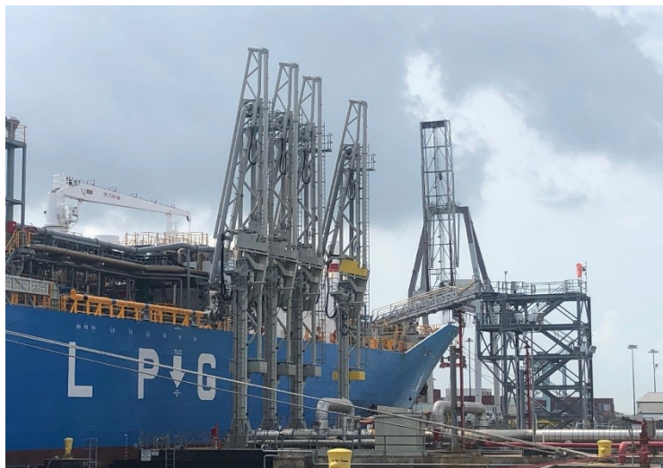
Loading arms – final testing
